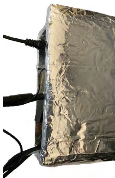
Picture 3 . Showing the receiver unit fully fitted into the Heat Proof pocket holder
