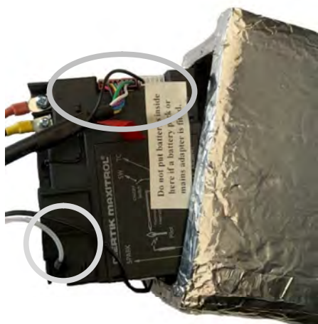
Picture 2 . Showing receiver unit being fitted into the Heat shield pocket . be careful not to pull any wires out of their multi-plug sockets as shown in the white circles
