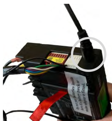
Pictures shows receiver unit with the Battery lead jack plug fitted . see white circle
